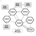
Fig. 3 IB Subnet Components
