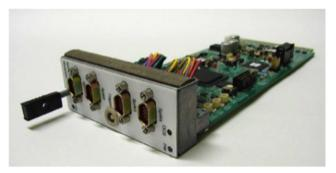
Figure 5. General-purpose SpaceWire Interface.
