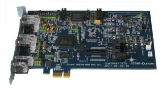
Figure 3 SpaceWire PCIe
