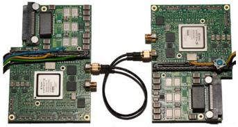
Figure 3: FPGA Testboards for Gigabit Communication with Comtronics CMRM cable
