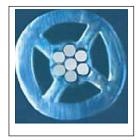
Fig. 1. Cross sectional view of an alveolar PTFE insulated conductor.
