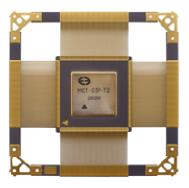
Fig. 2. MCT-03P with one gigabit port – the test sample of the MCT-03D chip without built-in silicon 4-channels gigabit router.
