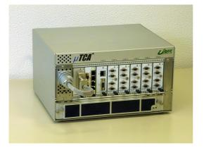
Fig.1 An example outlook of SpaceWire Traffic Generator enclosed in a 6-slot uTCA shelf. In this picture, 5 SpaceWire Traffic Generator modules are inserted, i.e. 20 external test ports are available. Two modules connected by a thick cable are power supply and distribution modules.
