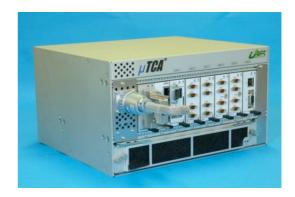
Figure 3. 6-slot SpaceWire backplane system using micro TCA system
