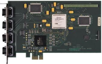
Figure 6 - SpaceWire acquisition board
