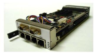
Figure 4. MCH with 28-port SpaceWire router.
